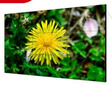
The DS-D2055HE-G LCD display uses an industry-level extreme-narrow bezel design, which enables a bezel width of 1.8 mm between neighboring displays. The adopted direct-lit LED backlighting technology helps achieve ultra-high and uniform brightness of 700 cd/m² without boundary shadows. The display has abundant interfaces for video inputs, such as DVI, VGA, HDMI, and DP.
