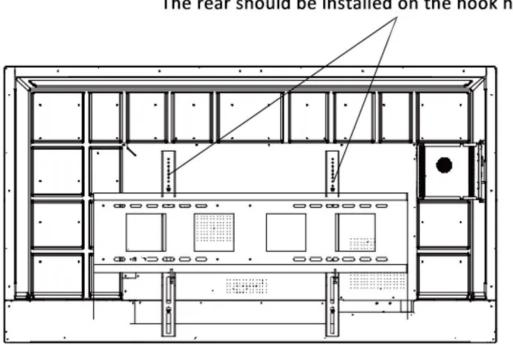
The rear should be installed on the hook holes
