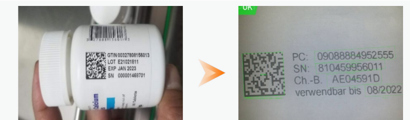
By using the AI method of OCR + code reading, up to more than 99.9% accuracy, it provides a more reliable and integrated solution for reading and identifying multiple information on the outer packaging of pharmaceutical boxes.
