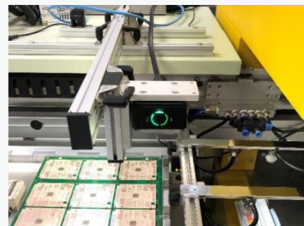
Multiple base color PCB board reading codes
