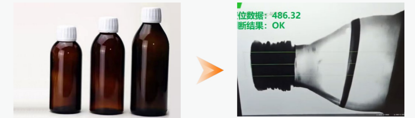
SC camera is compatible with a variety of product types and adaptive detection of a variety of liquid level heights, effectively avoiding air bubbles, impurities, etc. on the accuracy of liquid level detection.
