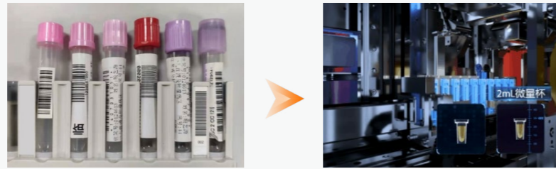
Arbitrary size, shape, label interference, blood color, etc. of the test tube does not affect the full autochemical detection of drug liquid test tube, the integrated camera can realize the sample container code identification, test tube category judgment, liquid level detection, etc.
