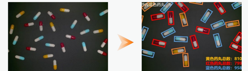
Under the high-speed application scenario, it accurately captures the information such as posture and shape of the real-time movement of materials, combines with AI algorithm, real-time analysis and processing, accurately calculates the number of materials, realizes real-time counting function, without fear of stacking and other problems, and foreign objects are automatically ignored.
