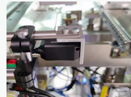
Silicon bar 2D code reading
