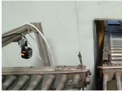
Automotive casting part code reading
