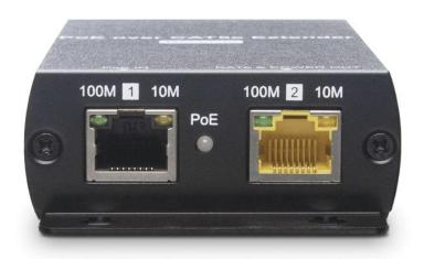
IPO9P is a point-to-point 800m long range PoE extender that uses a single ethernet cable (CAT5e, CAT6, CAT7) to transmit PoE signals. IPO9P supports IEEE 802.3 at, 802.3 af, 802.3 bt standard and provides up to 90W of power for a remote PoE device, which is ideal for a professional CCTV system to connect a remote PoE camera to a PoE switch in a plug-and-play installation.
