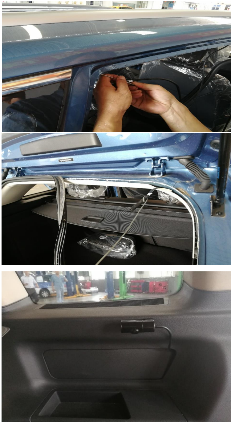
Figure 2-21 Run Cable by Iron Wire
