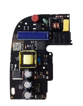
220V PSU for Hub/Hub 2/Hub 2 Plus/ ReX 2 Control panels
