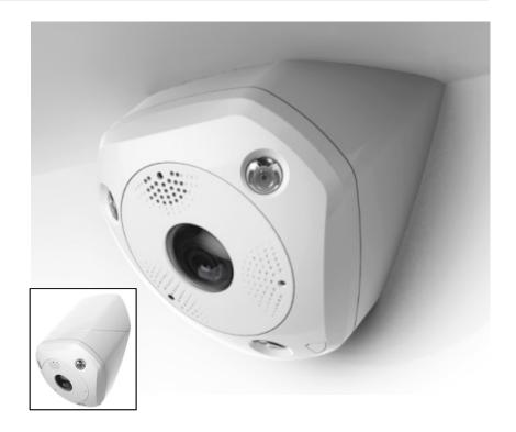
The Hikvision DS-2CD6W32FWD-IVS is designed to provide complete area coverage by eliminating blind spots below and to the side of the camera. The 3 MP progressive scan CMOS sensor, included 45° wall mount, and 2 mm panoramic lens provide 135° horizontal and 98° vertical fields of view.
