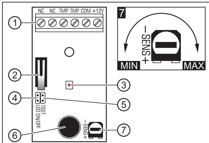
Fig. 1. View of the detector PCB.
