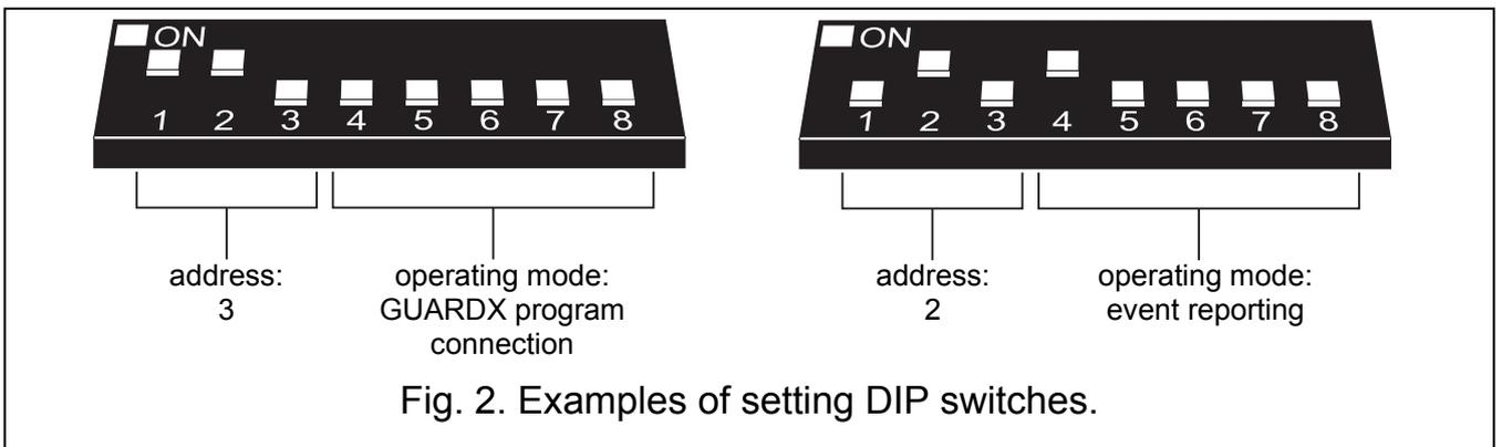
Fig. 2. Examples of setting DIP switches.
