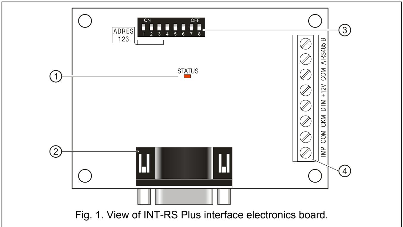
Fig. 1. View of INT-RS Plus interface electronics board.
