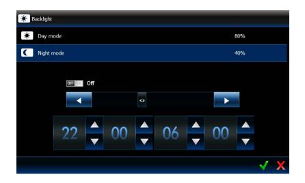
The screen backlight is adjustable and may be different depending on the time of day. Use the slider to set the brightness. If the night mode is to be used, turn on the appropriate option, and then specify the hours during which the night mode is to be used.
