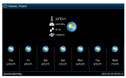
It presents weather and weather forecast. The data are downloaded from the OpenWeatherMap service (openweathermap.org). The installer sets the widget size, which determines for how many days the weather forecast will be presented.
