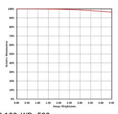
Note: The above curves are the simulate results based on F2.4,  $\beta$ =-0.109, WD=500 mm.
