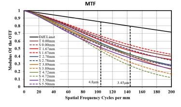
Note: The above curves are the simulate results based on F2.4,  $\beta$ =-0.039, WD=300 mm
