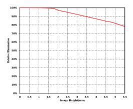
Note: The above curves are the simulate results based on F2.8,  $\beta$ =-0.076, WD=700 mm.
