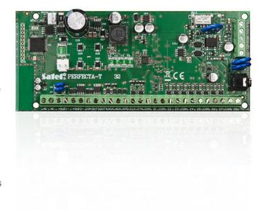
You can configure the system in two ways: by using the intuitive **PERFECTA Soft** program (from a computer connected with a RS–232 (TTL) cable) and by means of a keypad, using shortcut keys in the service menu.
