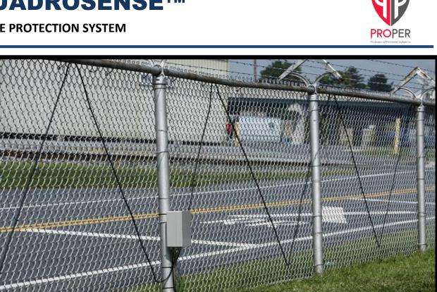
QuadroSense<sup>™</sup> is a special fence protection system. The main part of the system is the control unit, to which vibration sensitive **TB** cables are connected. The TB cable is a special triboelectric cable, which should be attached with cable tie to the fence to be protected, ideally in a saw-toothed or straight line pattern.
