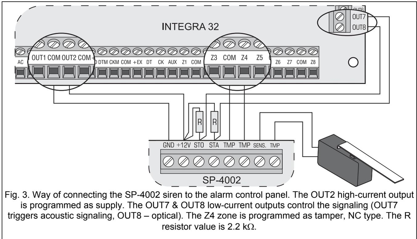
Fig. 3. Way of connecting the SP-4002 siren to the alarm control panel. The OUT2 high-current output is programmed as supply. The OUT7 & OUT8 low-current outputs control the signaling (OUT7 triggers acoustic signaling, OUT8 – optical). The Z4 zone is programmed as tamper, NC type. The R resistor value is 2.2 k $\Omega$ .
