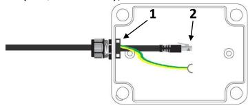
6. The other end is also connected to the RJ45 connector, and  $\frac{\text{make the nut locked into}}{(1)}$  into the waterproof set.
