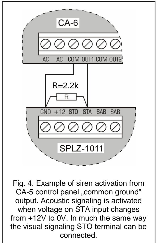
Fig. 4. Example of siren activation from CA-5 control panel „common ground” output. Acoustic signaling is activated when voltage on STA input changes from +12V to 0V. In much the same way the visual signaling STO terminal can be connected.
