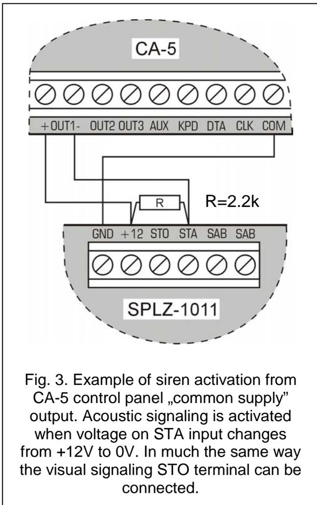
Fig. 3. Example of siren activation from CA-5 control panel „common supply” output. Acoustic signaling is activated when voltage on STA input changes from +12V to 0V. In much the same way the visual signaling STO terminal can be connected.
