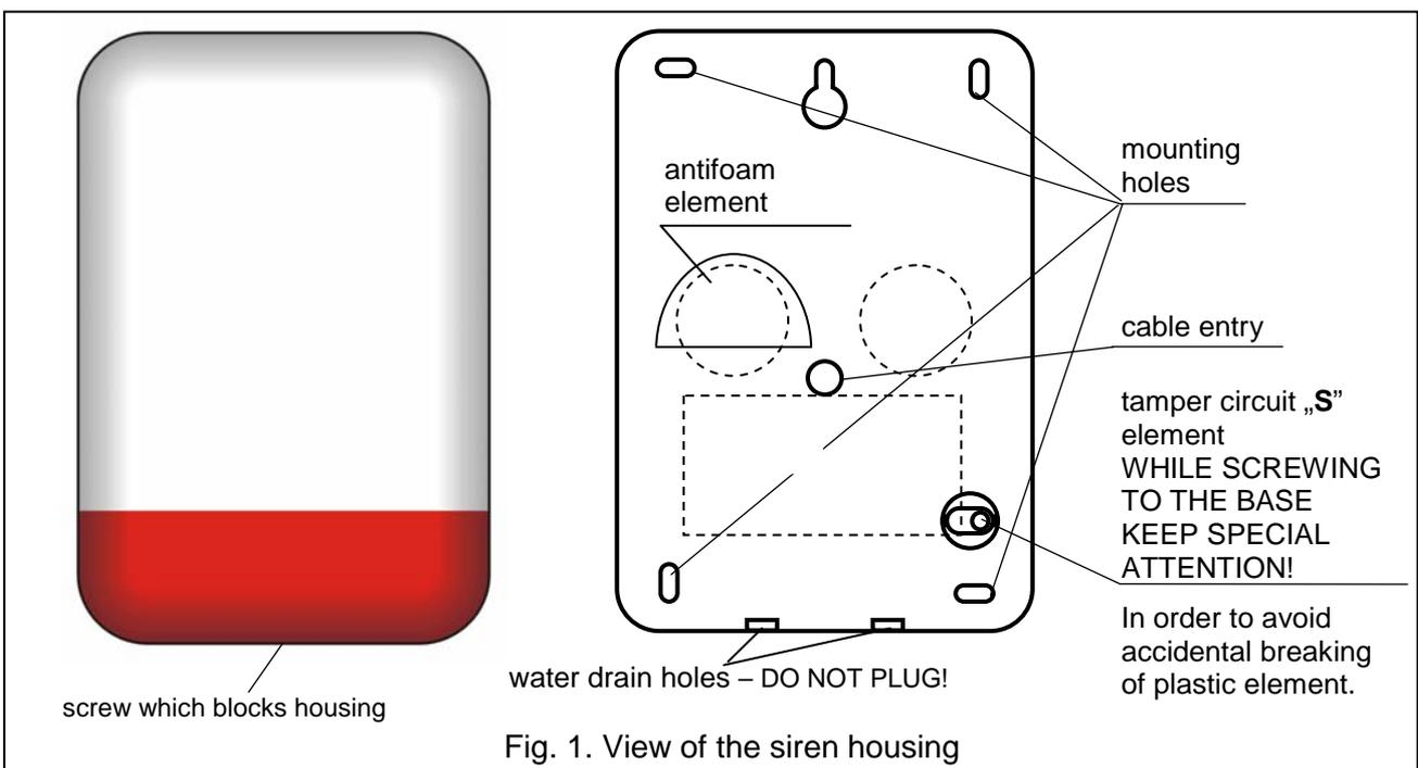
After installing the siren, it is recommended to seal the mounting holes and the cable entry with silicone compound.
